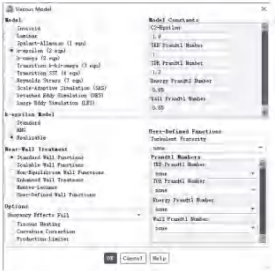
图 3 湍流模型的设置 Fig. 3 Setting of the turbulence model panel
